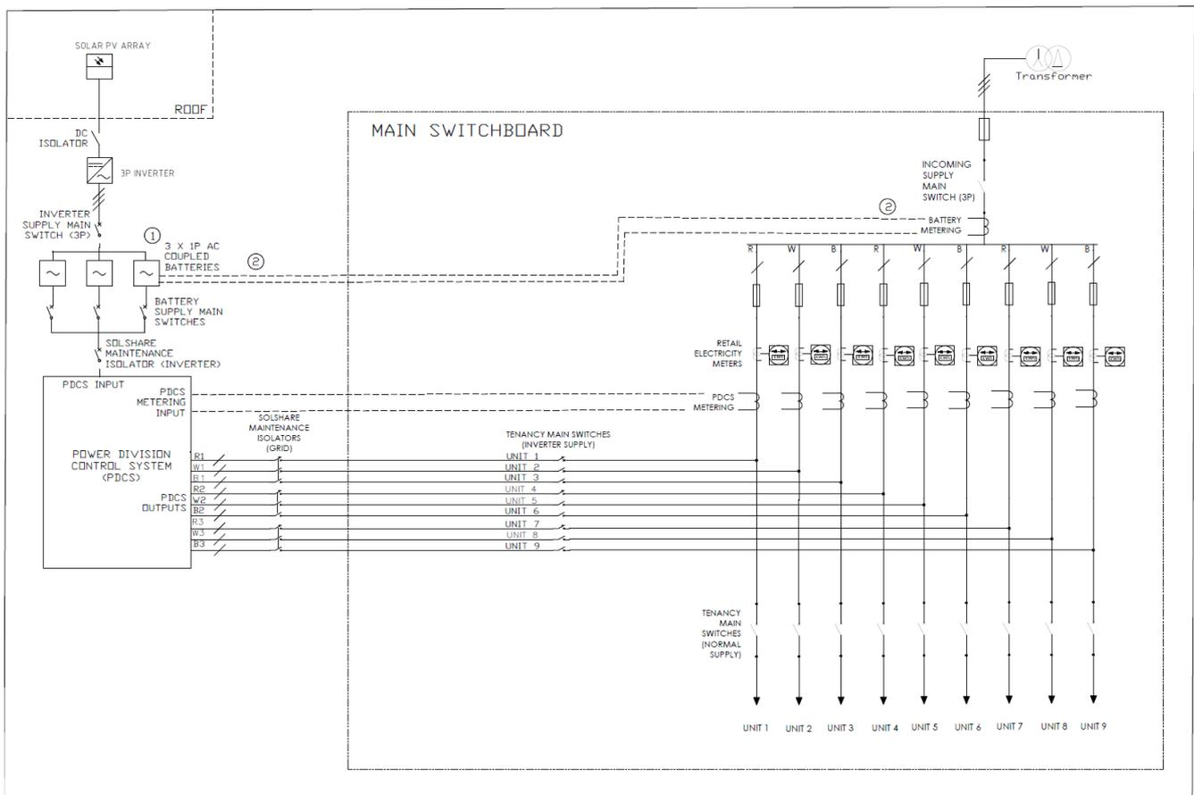
An example of an AC-coupled system with 3 x single phase batteries and a SolShare (utilising only 9 outputs)
