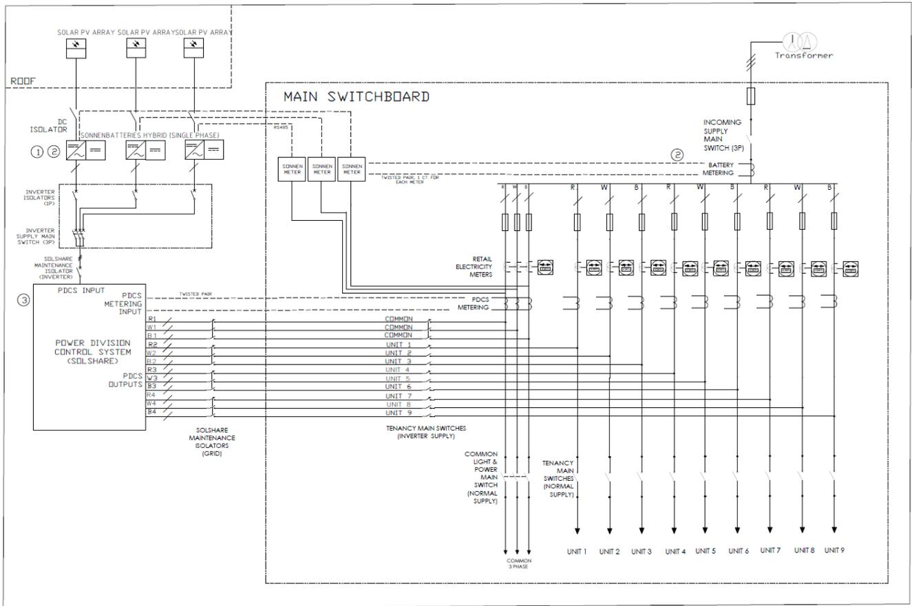
An example of a DC-coupled system with SolShare using Sonnen Batterie Hybrid batteries
