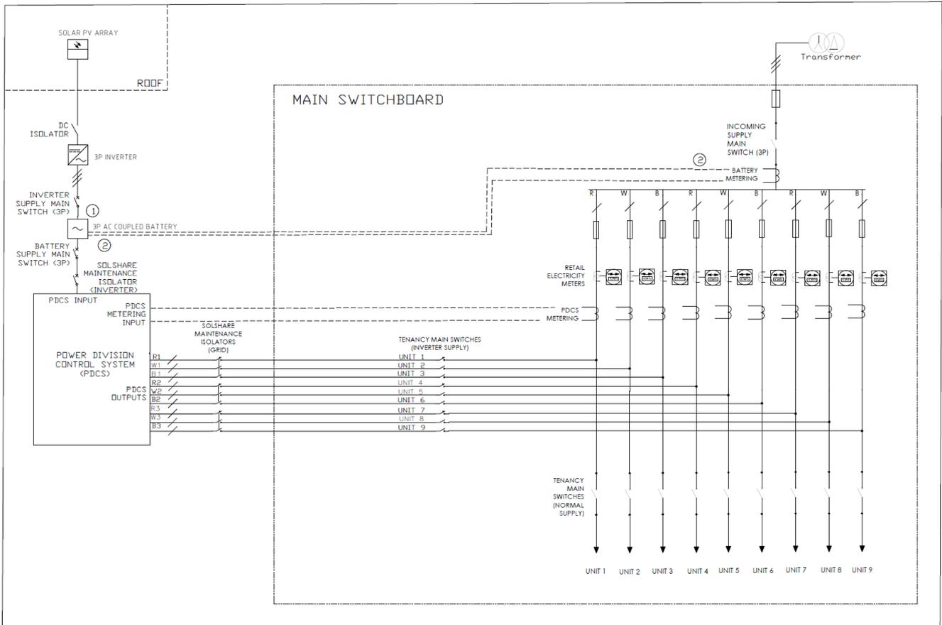
An example of an AC-coupled 3 phase battery system with SolShare (utilising only 9 outputs)
