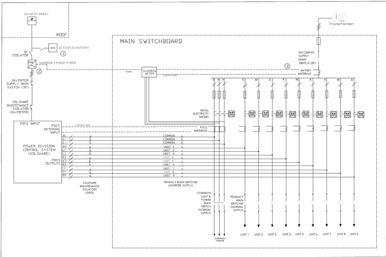
An example of a DC-coupled system with SolShare using a Sungrow battery
