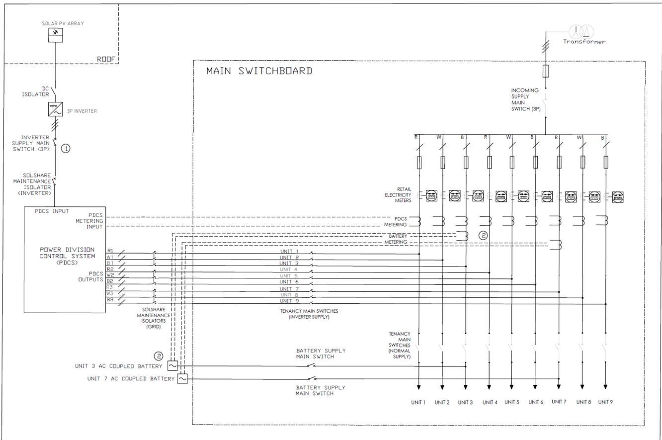
**6b: An example of 2 x AC-coupled batteries, each for a single tenancy – one used for Unit 3 and the other for Unit 7. The battery point of connection is between the Tenancy Main Switch (Normal Supply) and the tenancy.**
