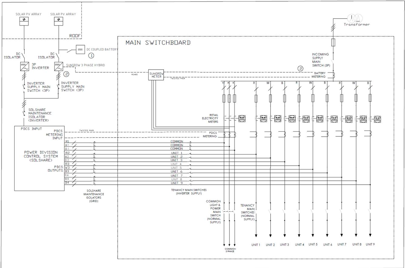
An example of a PV + separate PV/DC-coupled system with SolShare using a Sungrow battery
