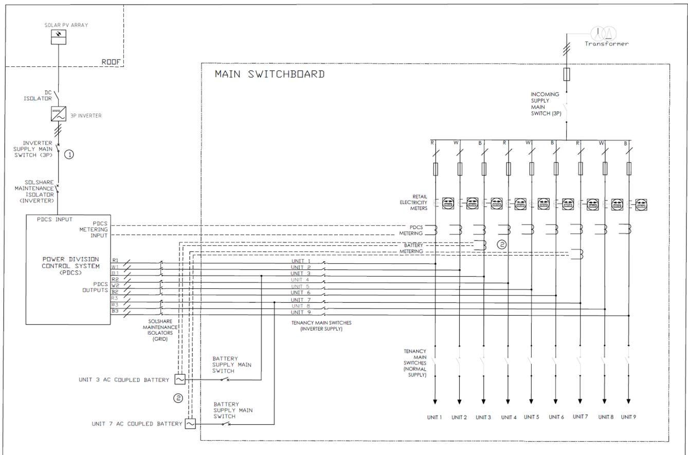
**6a: An example of 2 x AC-coupled batteries, each for a single tenancy – one used for Unit 3 and the other for Unit 7. The battery point of connection is between the maintenance isolator and the Tenancy Main Switch (Inverter Supply).**
