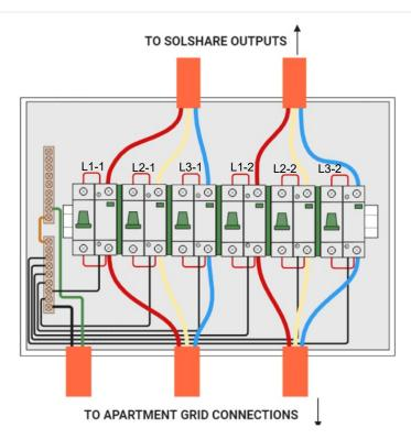
Only once all these isolators are open, along with the *Inverter Supply Main Switch*, will the SolShare be isolated.
